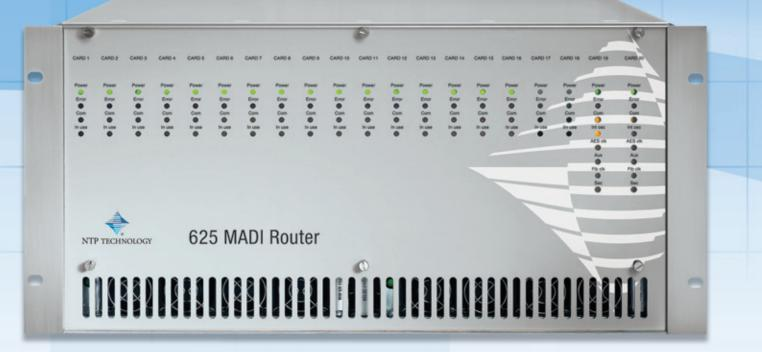
The NTP 625 MADI Router is a 2048<sup>2</sup> cross points router in a single 19" 5RU frame including dual controller and dual PSU. Up to 18 MADI cards with four MADI input and output interfaces can be installed.
